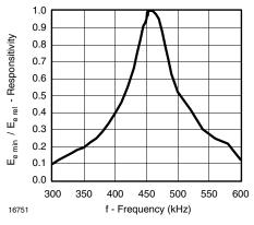
Figure 5. Frequency Dependence of Responsivity
