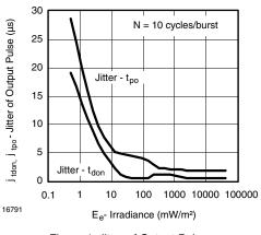
Figure 4. Jitter of Output Pulse
