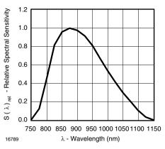
Figure 10. Relative Spectral Sensitivity vs. Wavelength
