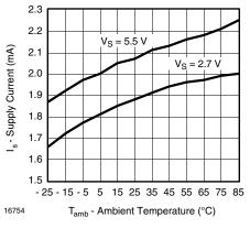
Figure 9. Supply Current vs. Ambient Temperature
