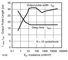
Figure 3. Output Pulse Diagram (t<sub>don</sub>, t<sub>po</sub>)
