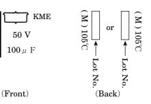
5 Manufacturer's identification mark 6Capacitance tolerance - (M) ⑦Lot No.
