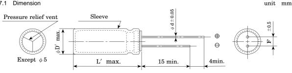
(Bottom view of gas escape end seal rubber)  $\phi 5 \sim \phi 10$
